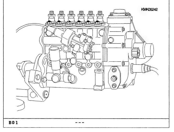
POSITIONER DISASSEMBLY Mount drive coupling on taper, drive end: RP 43 (taper 35 mm): - Taper length 28 mm: 1 686 430 038 1 686 430 040 - Taper length 36 mm: (Two-jaw version) RP 39 (taper 40 mm): 1 685 702 075 - Taper length 28 mm: - Taper length 41 mm: 1 685 702 076 (Flange version) Plus: - Hook wrench 1 687 950 530
